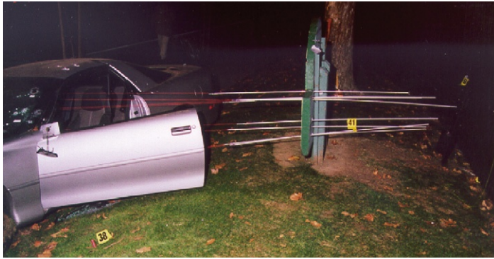
FIGURE 13.33 Brightly colored red string was used to extrapolate the paths of buckshot that passed through a wooden sign and continued into the vehicle while the door was in the open position. This reconstruction was conducted while the vehicle was in its original position at the scene.
