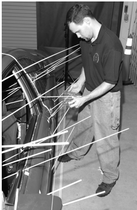
FIGURE 14.60 A protractor is employed to measure azimuth angles of various bullet paths represented by probes in this vehicle. Note the longitudinal reference line on the ground and a parallel reference line using string between two tripods that can be slid up and down to the various heights of the probes for convenient/accurate measurement with the protractor.
