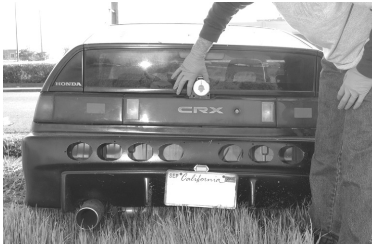
FIGURE 14.63 The lateral tilt of the vehicle is measured using an inclinometer at the scene to document its orientation relative to the terrain, which can later be used to correct estimated bullet paths determined after the vehicle is towed.
