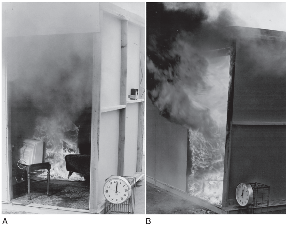
FIGURE 15.17 (A) Nonaccelerated fire in a furnished cubicle approaches flameover or rollover as the smoke layer begins to ignite into open flame. (B) Same fire 1 minute later: Radiant heat has ignited all furnishings and carpet throughout, completing the flashover transition. Postflashover fire is burning most intensely where ventilation (fresh air) supply is best. Note intense fire in the doorway.
