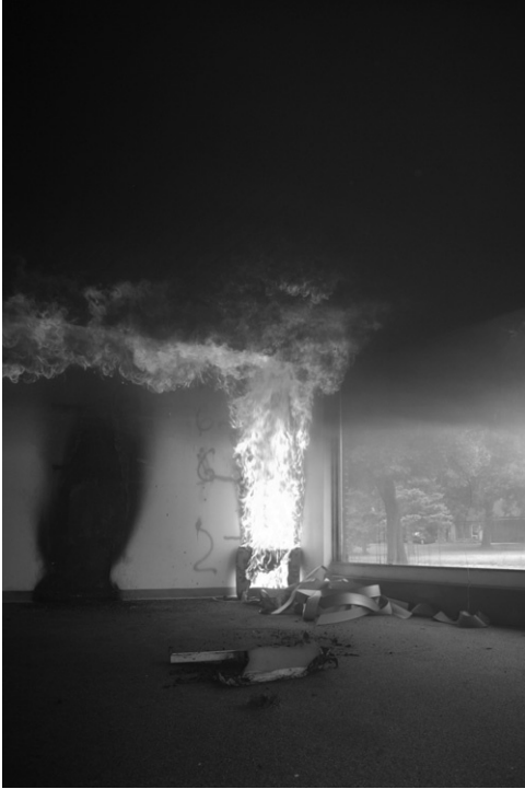
FIGURE 15.13 Chair fire producing a hot smoke (ceiling) layer in a room. Depending on the size of the room and size of vent openings (doors and windows) that can lose heat, the minimum size of the fire needed to trigger flashover can be calculated. Photo courtesy of Jamie Novak (Novak Investigations, Lindstrom, MN).
