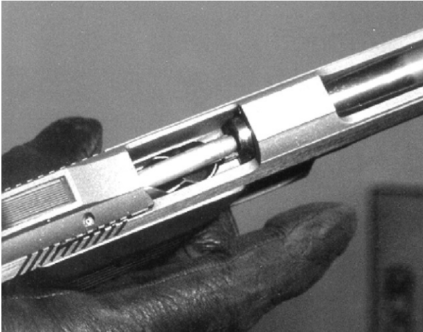
FIGURE 13.7 This close-up photo, taken by an astute police officer, documents a jammed cartridge in the chamber of the pistol. This key form of documentation corroborated statements made by witnesses that the suspect pointed the gun at police officers but failed to fire the gun.
