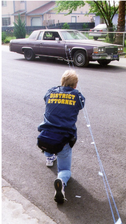
FIGURE 13.34 This photograph illustrates the bullet path from the perspective of the shooter. Colored strings with colored Post-It notes attached at 2-foot intervals for increased visibility in the photograph represent these two bullet paths.
