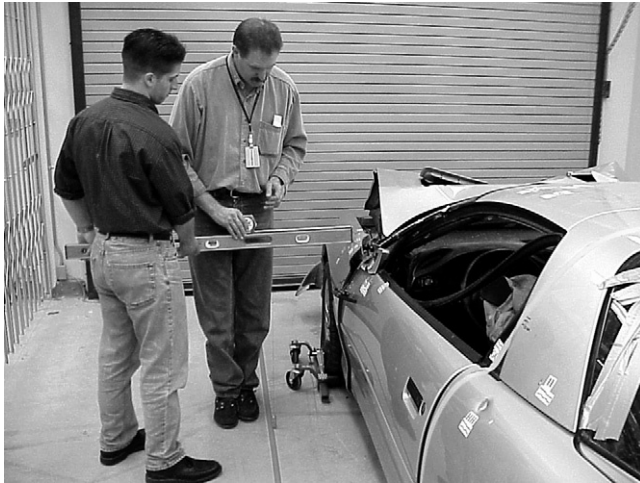
FIGURE 14.59 A 4-foot level, measuring tape, and plumb bob are used to accurately plot the location of bullet holes using the reference line. Measurements taken using this method can generate accurate scaled computer-aided design (CAD) diagrams of the bullet paths through the vehicle that can be imported into other scaled CADs of the shooting scene.
