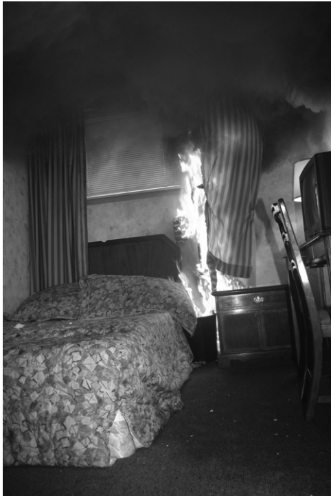
FIGURE 15.16 Vertical fire growth on bedding and draperies (from wastebasket) is very rapid. The depth and temperature of the hot smoke layer will both increase rapidly. Photo courtesy of Jamie Novak (Novak Investigations, Lindstrom, MN).
