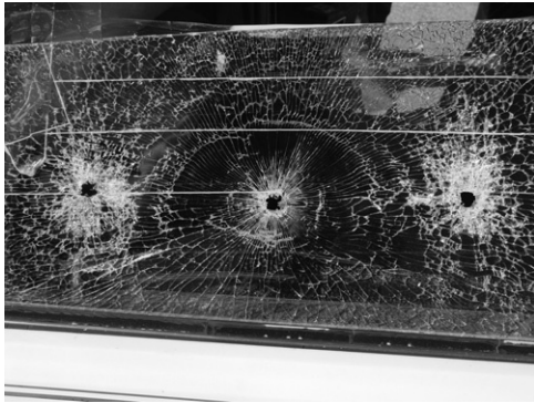
FIGURE 13.15 Radial fractures surrounding the bullet hole in the center of this tempered glass automobile window indicate damage from the first bullet that passed through it. The two remaining bullet holes exhibiting an absence of radial fractures and surrounded by classic cube/rectangular-shaped fractures were subsequently produced. However, it is not possible to sequence them further due to the dynamics of tempered glass fracture behavior.
