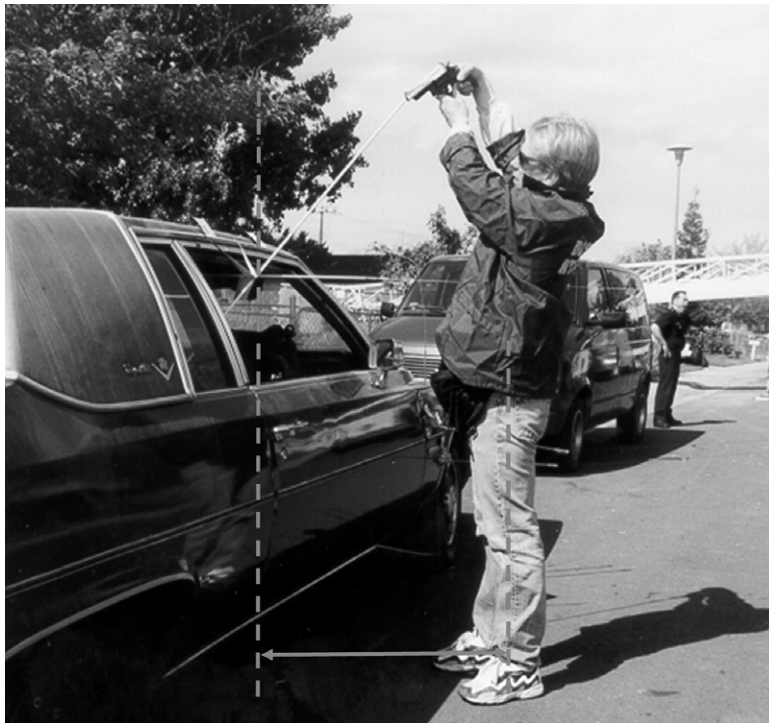
FIGURE 13.45 Impossible: Any distance equal to or greater than the distance represented by the arrow is reported as the zone of impossibility, as the shooter is no longer able to place the firearm in alignment with the reconstructed bullet path.
