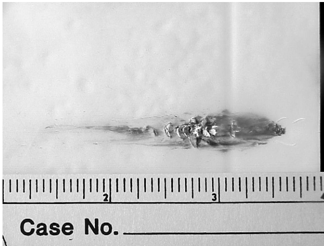
FIGURE 13.26 A lead bullet deflecting off of a linoleum floor surface traveling from right to left at 20 degrees produced this ricochet mark. Note that the asymmetrical extension of the graze mark favoring the lower edge, termed the Chisum trail, is caused by the left edge of the impacting bullet remaining in contact with the surface after the main body of the bullet has lifted off the surface while rotating in a counterclockwise direction from the left twist rifling of the firearm that fired it. If the asymmetry were extended to the upper side, it would indicate a right twist rifled barrel. This indicator of rifling twist direction could potentially be used to include or exclude the involvement of candidate firearms in a shooting incident.
