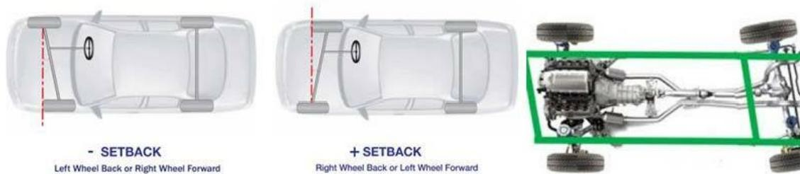
**“Thrust angle”** is the angle between vehicle longitudinal geometrical center line and line from the mid-point between the two rear wheels (thrust line).
