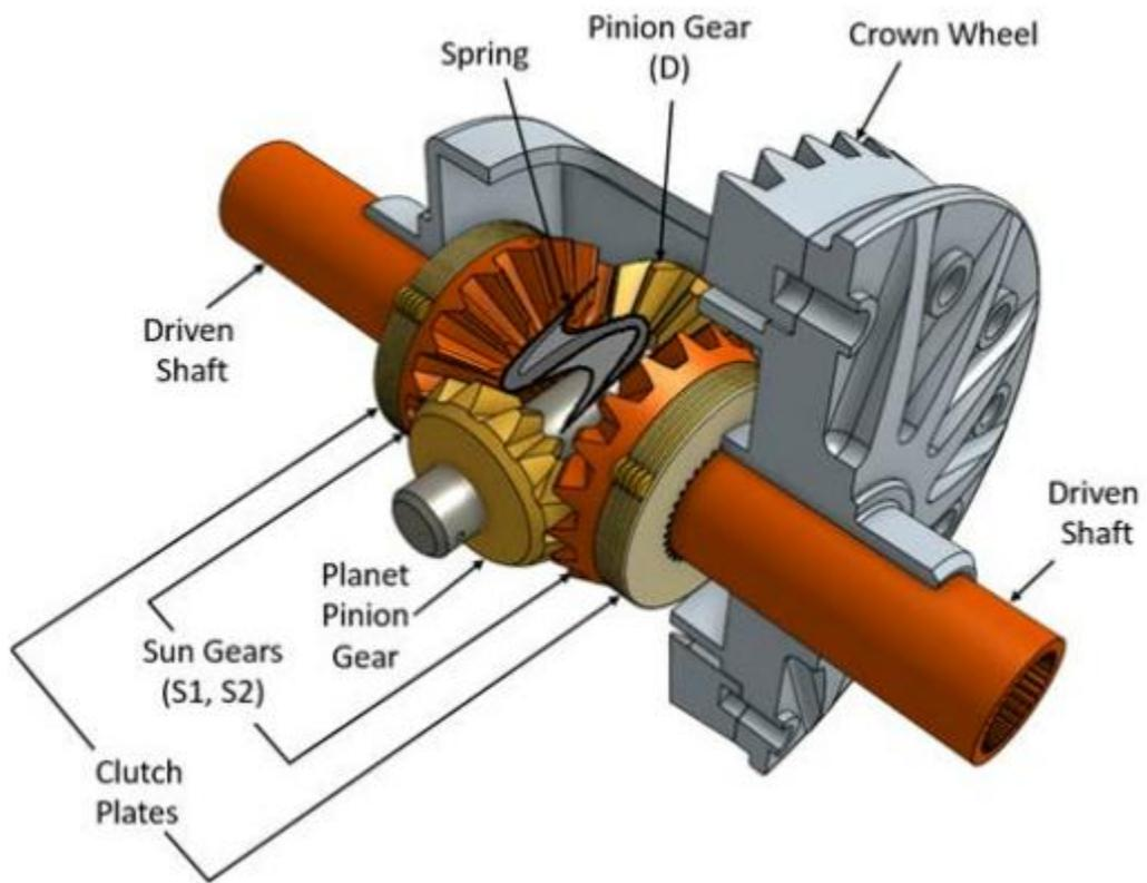
**VIDEO OF WORKING PRINCIPLE OF CLUTCH TYPE LIMITED SLIP DIFFERENTIAL**
