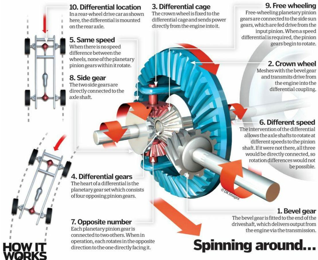
During movement of the vehicle on straight, level road and with both tires having equal traction (traction means adhesive or pulling friction of a tire on the road), there is no differential action. In this case, the crown wheel, differential case and cover, differential pinion gears and the differential sun gears all turn as one unit. The differential pinion gears do not rotate about their axis on the spider but rather turn both the sun gears and axle shafts at the same speed.
