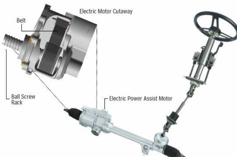
Pictures above shows the construction and operation of an electric power assisted steering mechanism.
