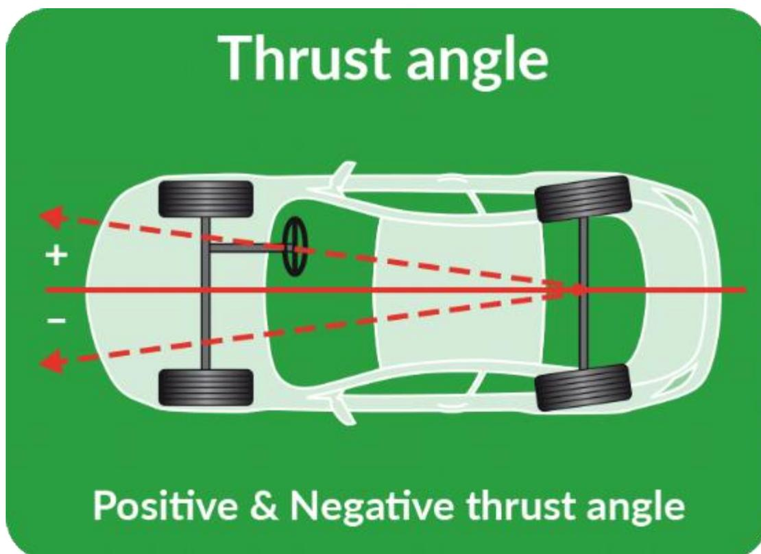
Figure below recapitulates some of the steering geometry parameters viewed from various positions in the vehicle: -
