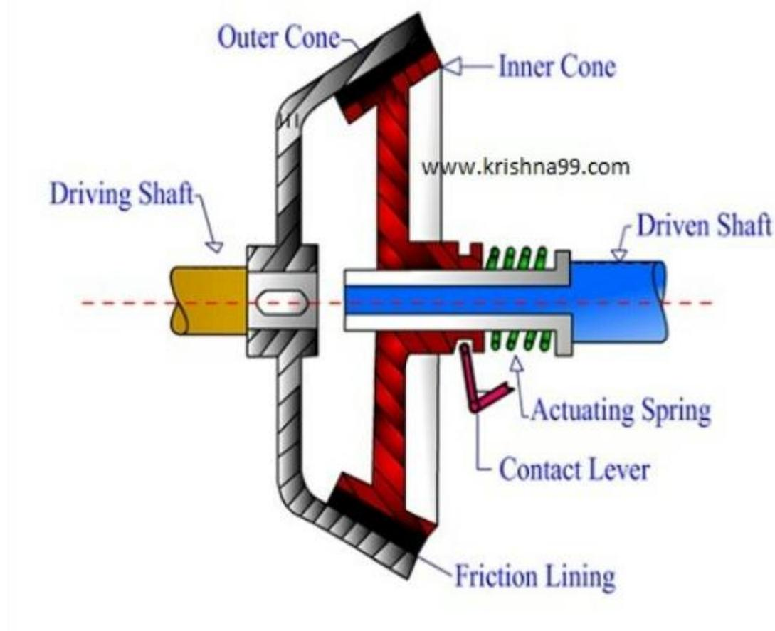
The engine shaft consists of a female cone, the male cone can slide on the clutch shaft. When the clutch is engaged the friction surfaces of the male cone is in contact with that of the female cone due to the force of spring. When the clutch pedal is pressed, the male cone slides against the spring force and the clutch is disengaged.
