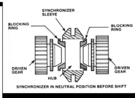
The arrangement and functions of various components of a typical synchronesh gearbox is mentioned below: -
