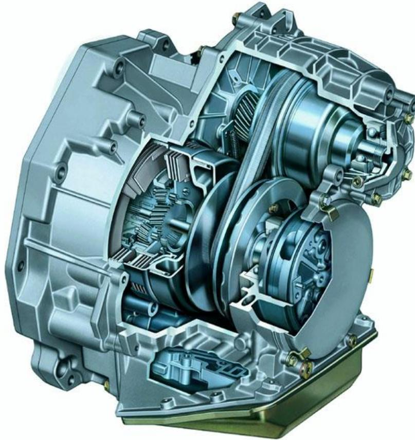
**VIDEO OF WORKING OF A CONTINUOUSLY VARIABLE TRANSMISSION**
