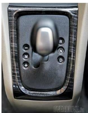
R: Reverse, N:Neutral, D: Drive, M: Manual, +/- : Gear shift in Manual mode
