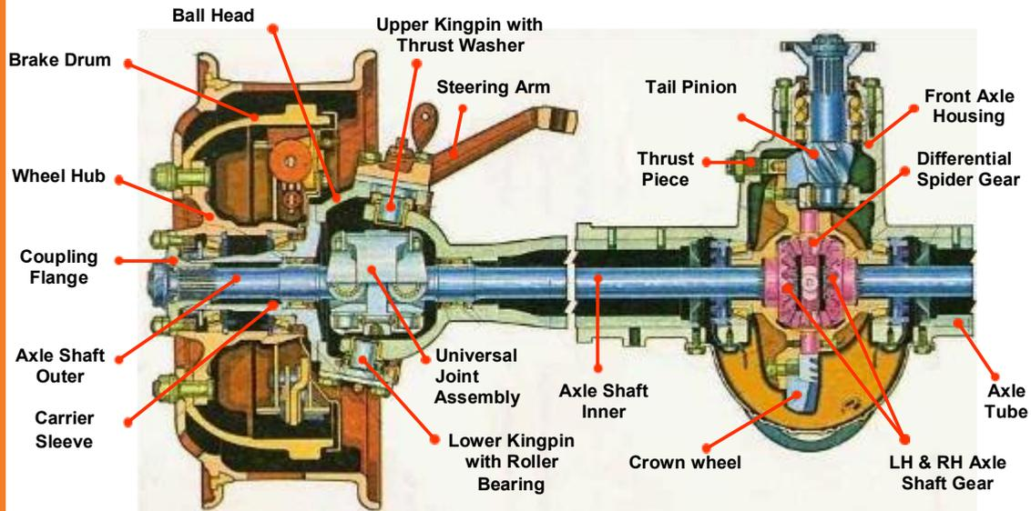
The front axles are generally dead axles, which does not transmit power. The front wheel hubs rotate on antifriction bearings of tapered-roller type on the stub axles. To permit the wheels to be turned by the steering gear, the steering spindle and steering knuckle assemblies are hinged on the end of the stub axles. The pin that forms the pivot of this hinge is known as king pin or steering knuckle pin.
