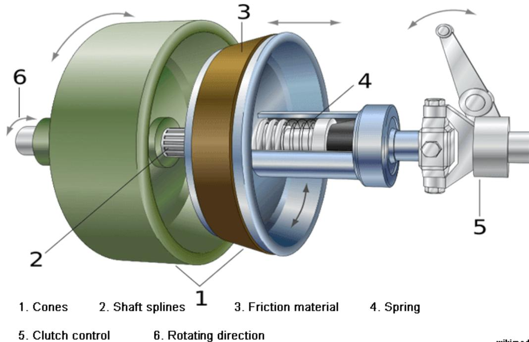
• **Principle of Operation of Centrifugal Clutch: -**
