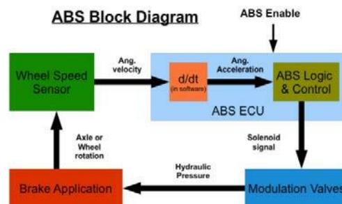
The ABS system comprises of **four main components** as below: -
