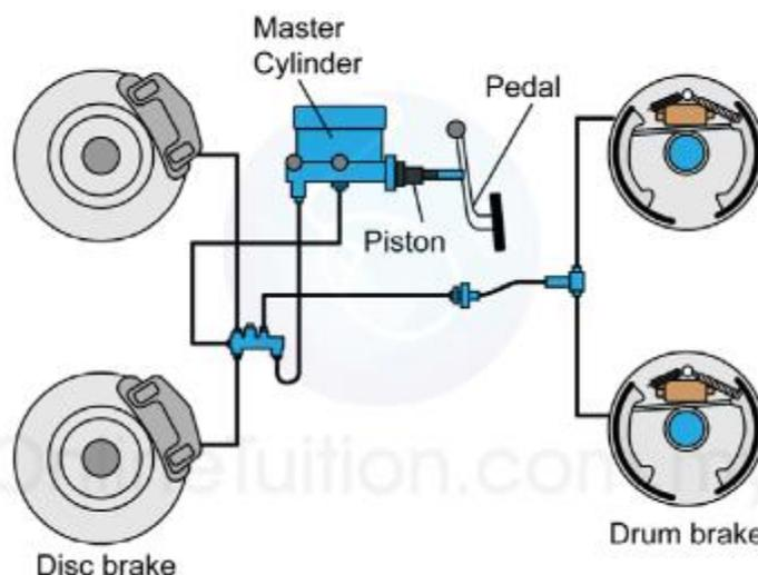
A hydraulic braking system transmits brake-pedal force to the wheel brakes through pressurized fluid, converting the fluid pressure into useful work of braking at the wheels. Layout of a hydraulic braking system having disc brakes in front wheels and drum brakes in rear wheels is shown above.
