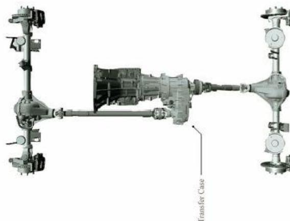
The typical transfer case is attached to the rear of the transmission in place of the extension housing. Engine power flows through the transmission output shaft to the transfer case input shaft. If the vehicle has *part-time four-wheel drive*, the driver selects either 2WD or 4WD mode. Gearing in the transfer case then sends power to only the rear axle (2WD mode) or to both front and rear axles (4WD mode).
