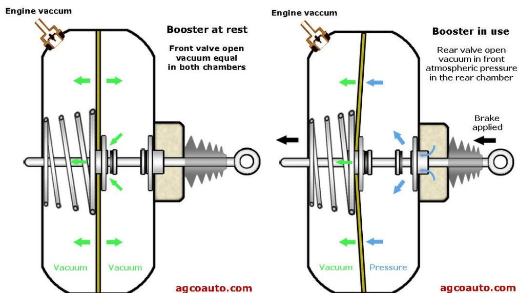
Schematic layout of a vacuum brake booster is shown above.
