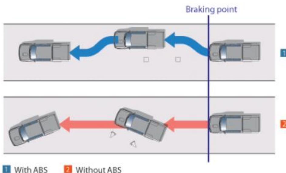
It is difficult to assess the required brake pedal force to be applied for an emergency stop in the shortest possible distance. This is because it is practically impossible to consider several varying factors such as: -
