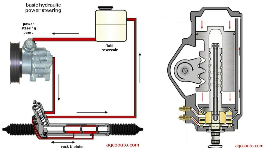
Picture on left above shows a **“Hydraulic assisted Rack and Pinion steering”** while that on the right shows a **“Hydraulic assisted Recirculating Ball type steering”**. Both use hydraulic power to boost the steering effort by the driver.
