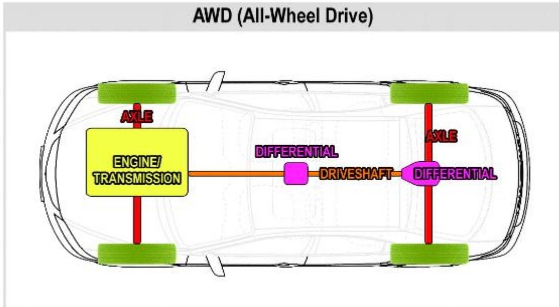
Other AWD vehicles have front-wheel drive with auxiliary rear-wheel drive, or rear-wheel drive with front wheel drive. Some AWD vehicle have a single speed transfer case. Others have the gearing to drive the auxiliary axle built into the transmission or transaxle.
