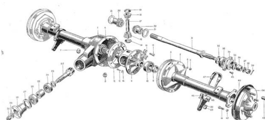
Fig. J.1. REAR AXLE—COMPONENTS.
