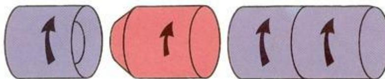
*Two conical surfaces are brought together, the friction between them causing the speed to synchronize.*
