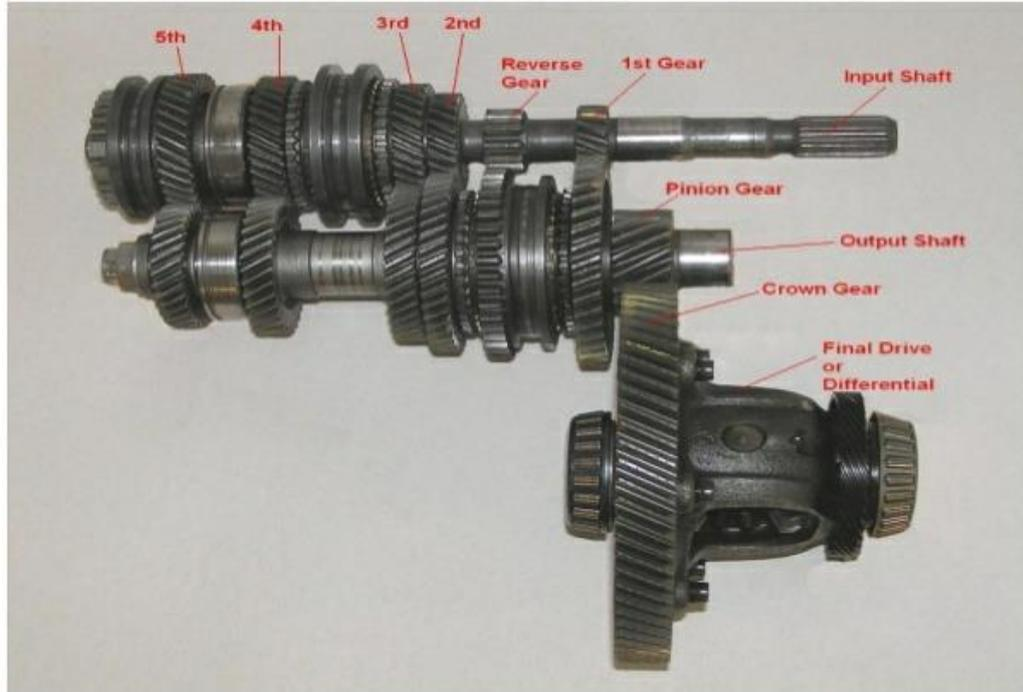
The power flow through the transmission section of the transaxle is the same as through a conventional transmission.
