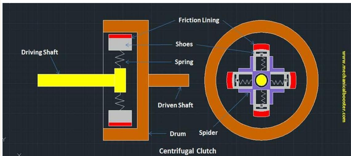
Main parts of a Centrifugal clutch are: -
