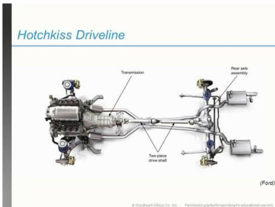
The arrangement uses two rear leaf springs, which are longitudinally mounted and are connected to the chassis frame by a “fixed” pivot at the front and swinging shackles at the rear. A universal joint is mounted at each end of the exposed or “[Open type Propeller shaft](#)” with provision for accommodating change in shaft length due to the deflection of the springs through a slip joint.
