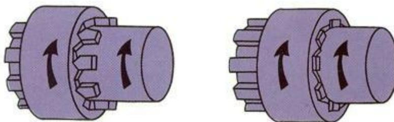
*As the collar slides along the shaft, it engages with the pointed splines, aligning them as it does so, and locks the two shafts together; in the more effective baulk-ring system and intermediate ring prevents engagement of the gears before speeds have been synchronised.*
