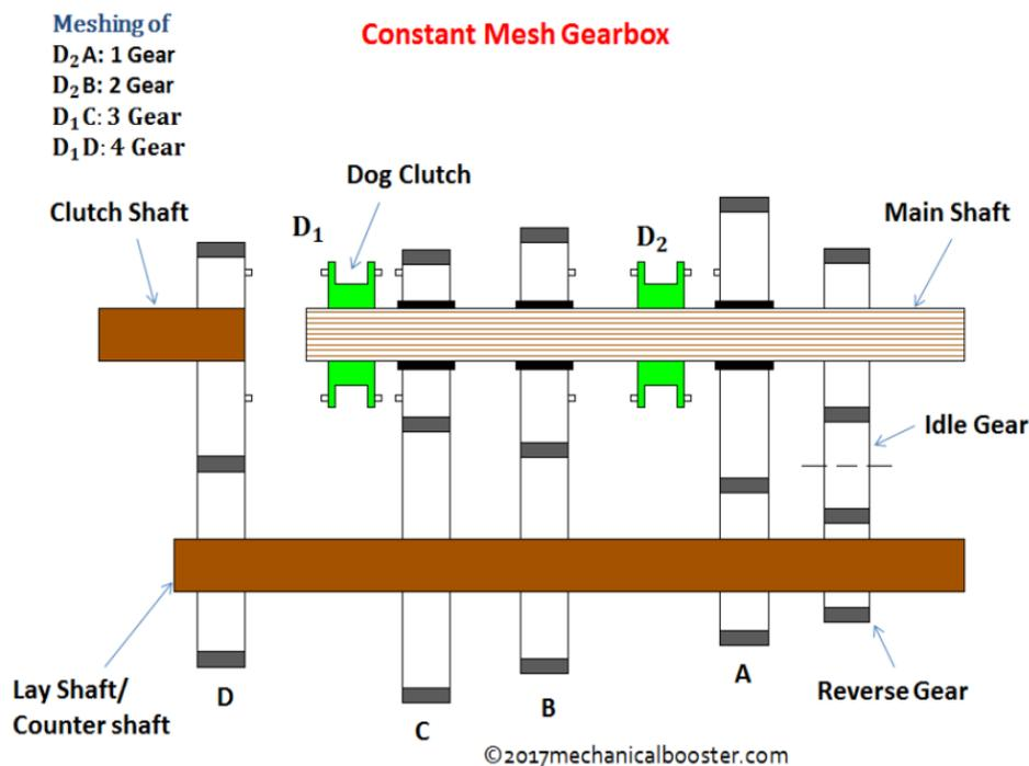
The construction or main components of constant mesh gearbox are:
