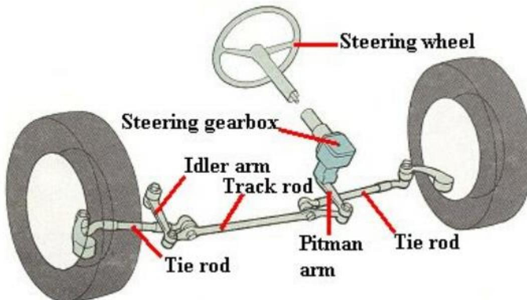
The steering system allows the driver to control the direction of vehicle travel. This is made possible by linkages that connects the *steering wheel* to the steerable wheels and tires. To increase the mechanical advantage of the rotary motion of the steering wheel to liner motion, a *steering gear box* is provided between the steering wheel and the linkages as shown above.
