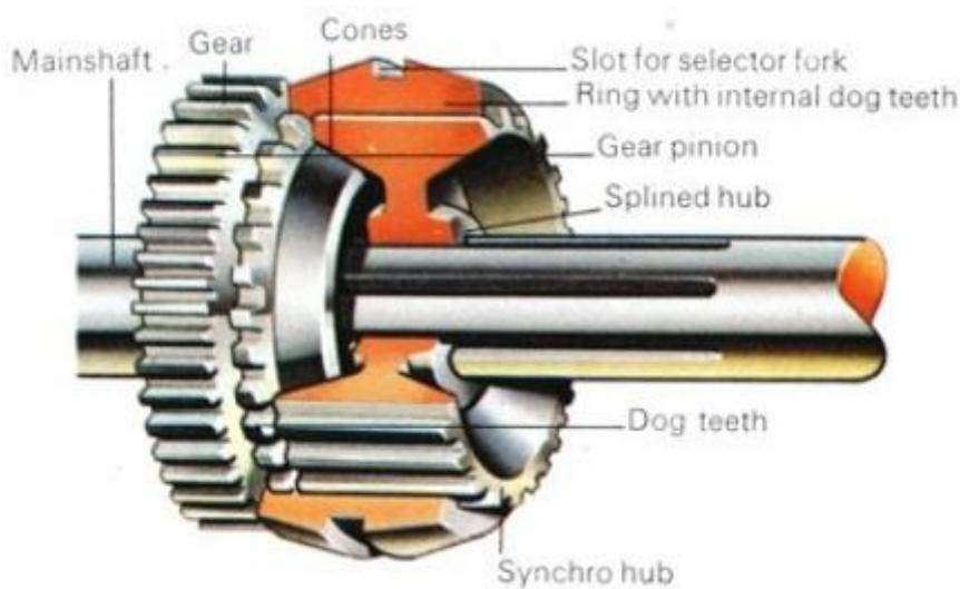
*Friction from the contact of the cones synchronizes their speed and the dog teeth slide into mesh to lock the gear and shaft.*
