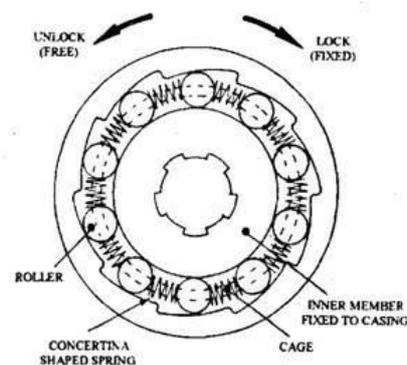
A more sophisticated and rugged design has spring-loaded steel rollers inside a driven cylinder. Rotating in one direction, the rollers lock with the cylinder making it rotate in unison. Rotating slower, or in the other direction, the steel rollers just slip inside the cylinder.
