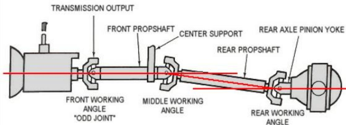
This shaft must be strong to resist the twisting action of the driving torque and it should be resilient to absorb the torsional shocks. It must resist the natural tendency to sag under its own weight because vibration occurs when the centre of gravity does not coincide with the axis of the shaft.
