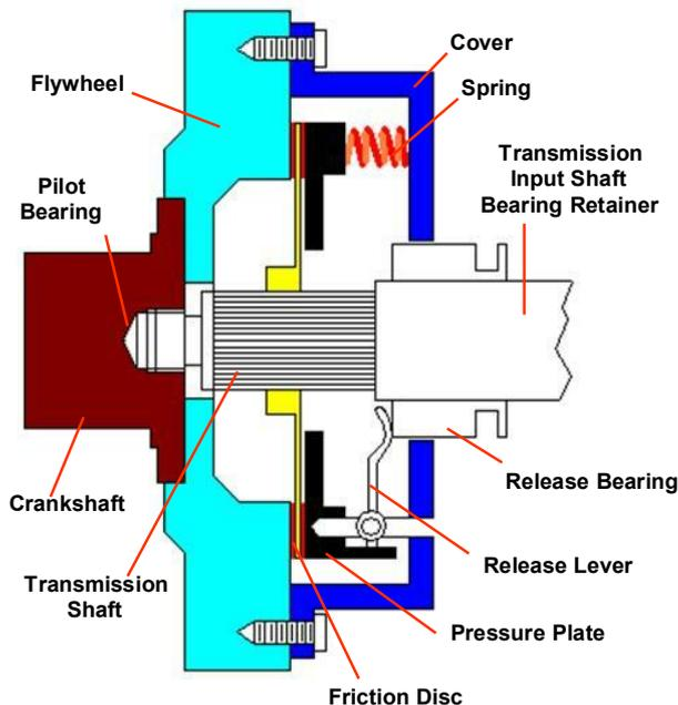
• The clutch consists of three main parts –
