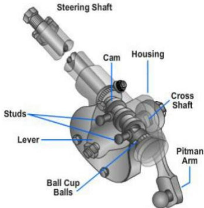
○ **Worm and Roller Type Steering Gear Box:**
