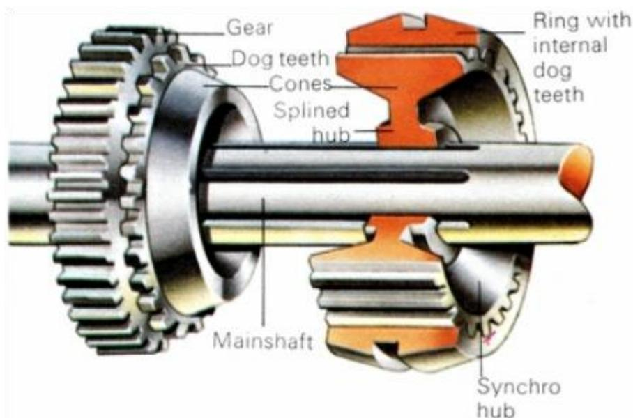
*The job of the synchromesh is to synchronize the rotational speeds of the gear and main shaft before locking them together.*
