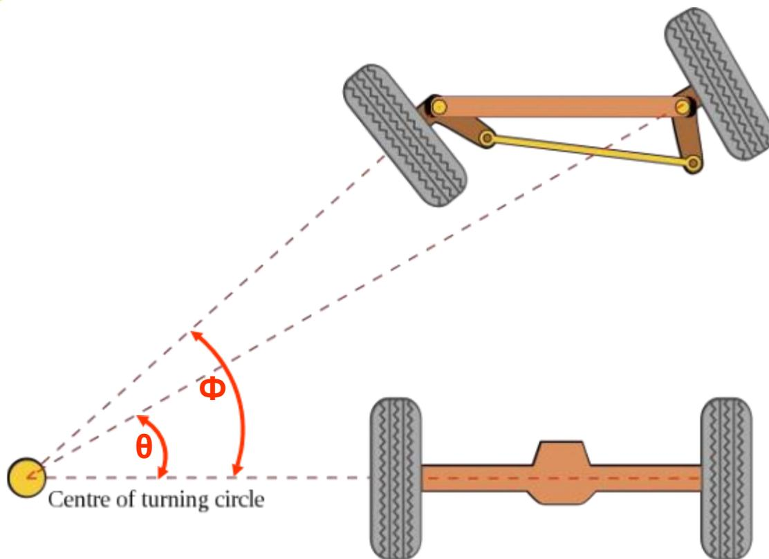
In order to avoid tire slippage when a vehicle takes a turn, it is necessary that each wheel must roll on an arc which has a common center with arcs of other wheels of the vehicle as shown above. This condition is called as “Pure rolling”. To satisfy the situation of pure rolling, following conditions must be satisfied: -
