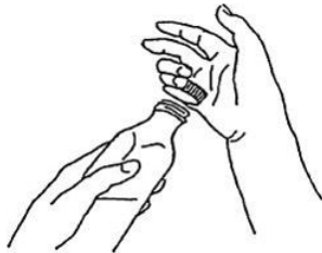
Figure 1-1a. Aseptically removing a bottle cap, freeing the rest of the hand to manipulate a plate lid, pipette, etc.
