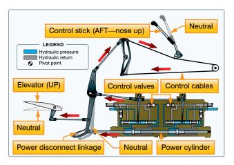
Figure 6-2. Hydromechanical flight control system.
