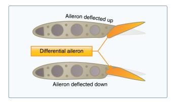
Figure 6-6. Differential ailerons.
