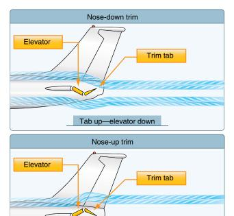
**Figure 6-20.** The movement of the elevator is opposite to the direction of movement of the elevator trim tab.
