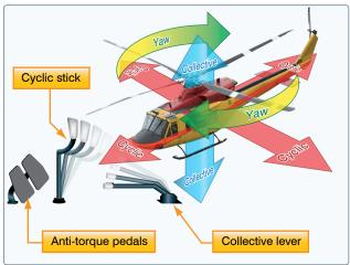
Figure 6-3. Helicopter flight control system.
