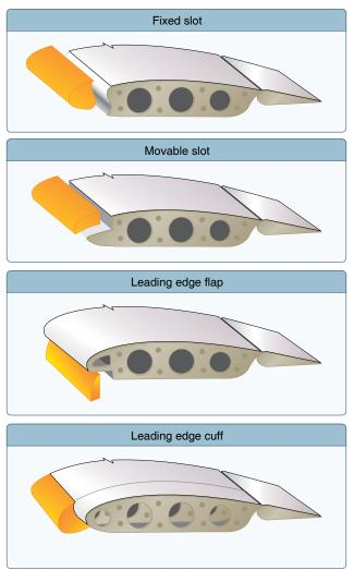
Figure 6-18. Leading edge high lift devices.
