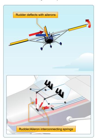
Figure 6-8. Coupled ailerons and rudder.
