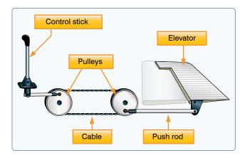
Figure 6-1. Mechanical flight control system.
