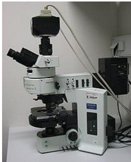
Fig: An upright fluorescence microscope (Olympus BX61)
