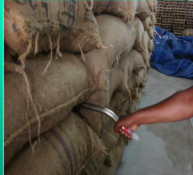
b) Placement of stack probe trap
