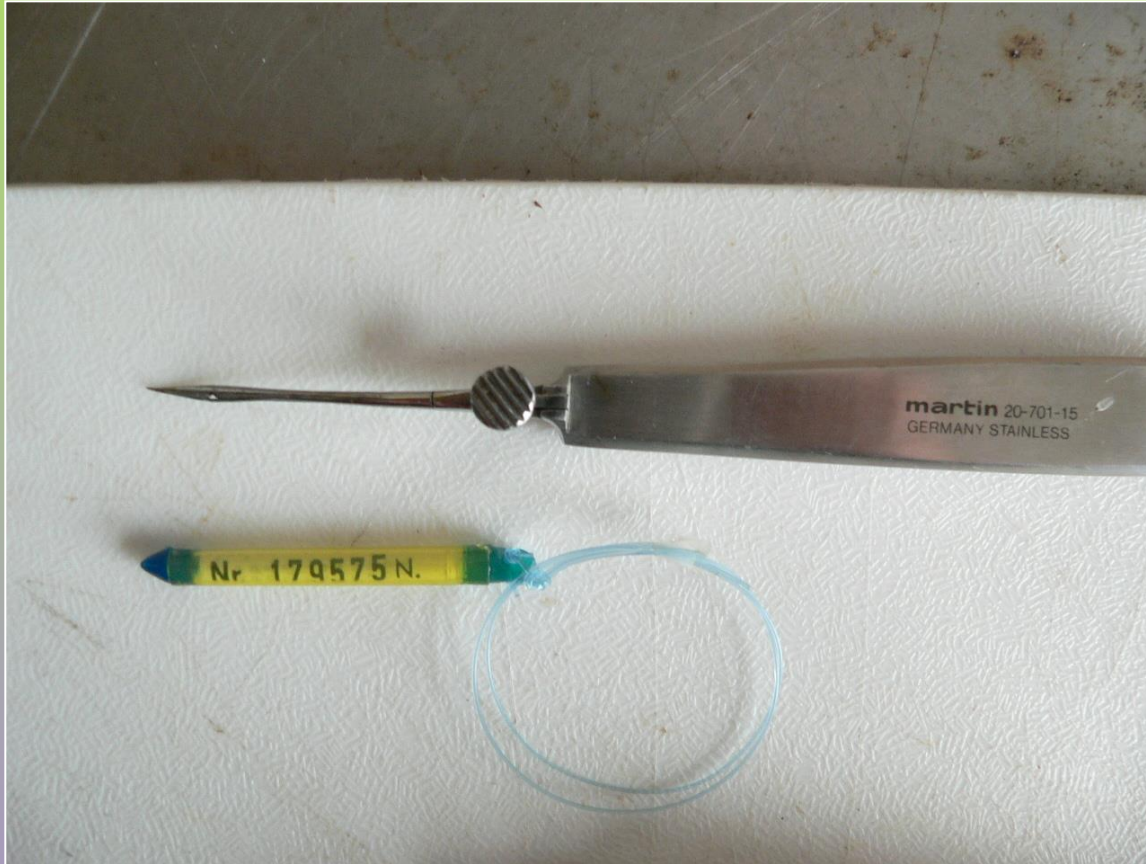
Tagging needle and Lea hydrostatic tag
