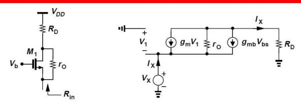
From the small-signal equivalent circuit for finding input impedance, we have
