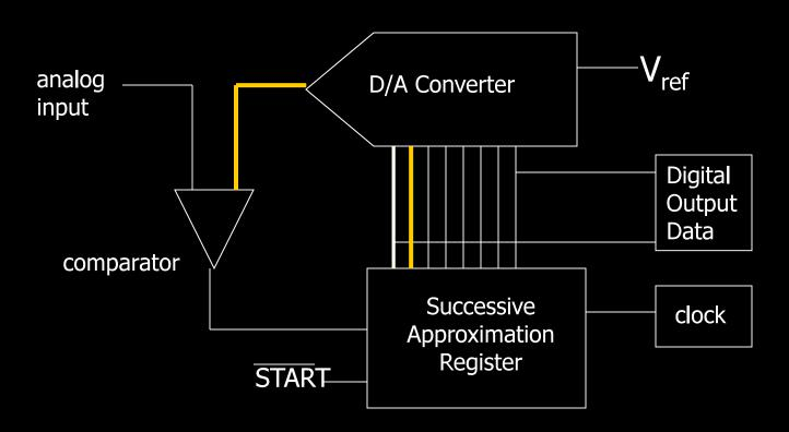
If the Vin < converted MSB then the MSB is left at 1 and the next bit is then tested.
