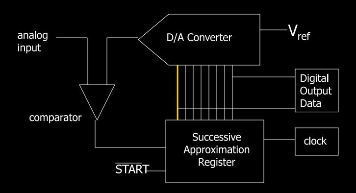
First the logic circuit in the SAR sets the MSB bit equal to 1 (+5 V). The MSB representing one half of full scale is converted by D/A converter.
