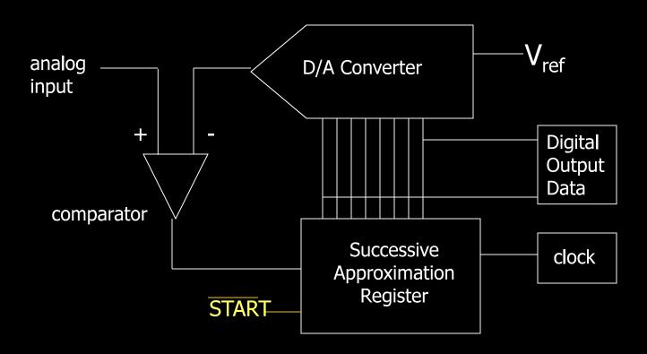
At initialization, all bits from the SAR are set to zero(clearing), and conversion begins by taking START line low.
