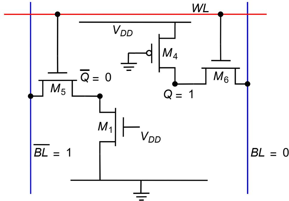
$$k_{n, M6} \left( (V_{DD} - V_{Tn}) V_Q - \frac{V_Q^2}{2} \right) = k_{p, M4} \left( (V_{DD} - |V_{Tp}|) V_{DSATp} - \frac{V_{DSATp}^2}{2} \right)$$
