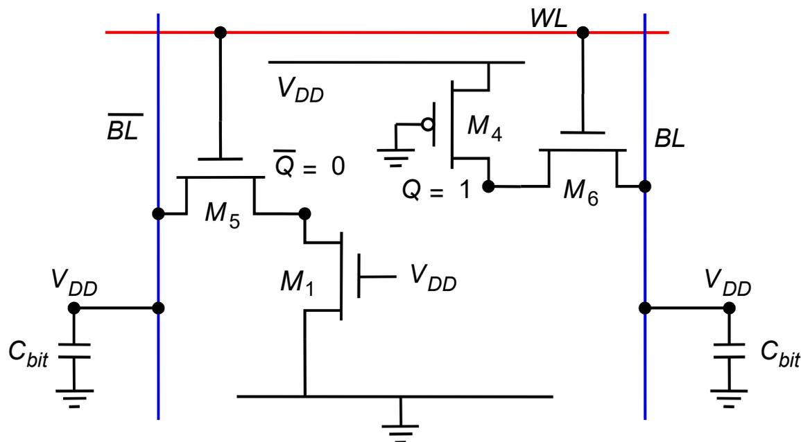
$$k_{n,M5} \left( (V_{DD} - \Delta V - V_{Tn}) V_{DSATn} - \frac{V_{DSATn}^2}{2} \right) = k_{n,M1} \left( (V_{DD} - V_{Tn}) \Delta V - \frac{\Delta V^2}{2} \right)$$
