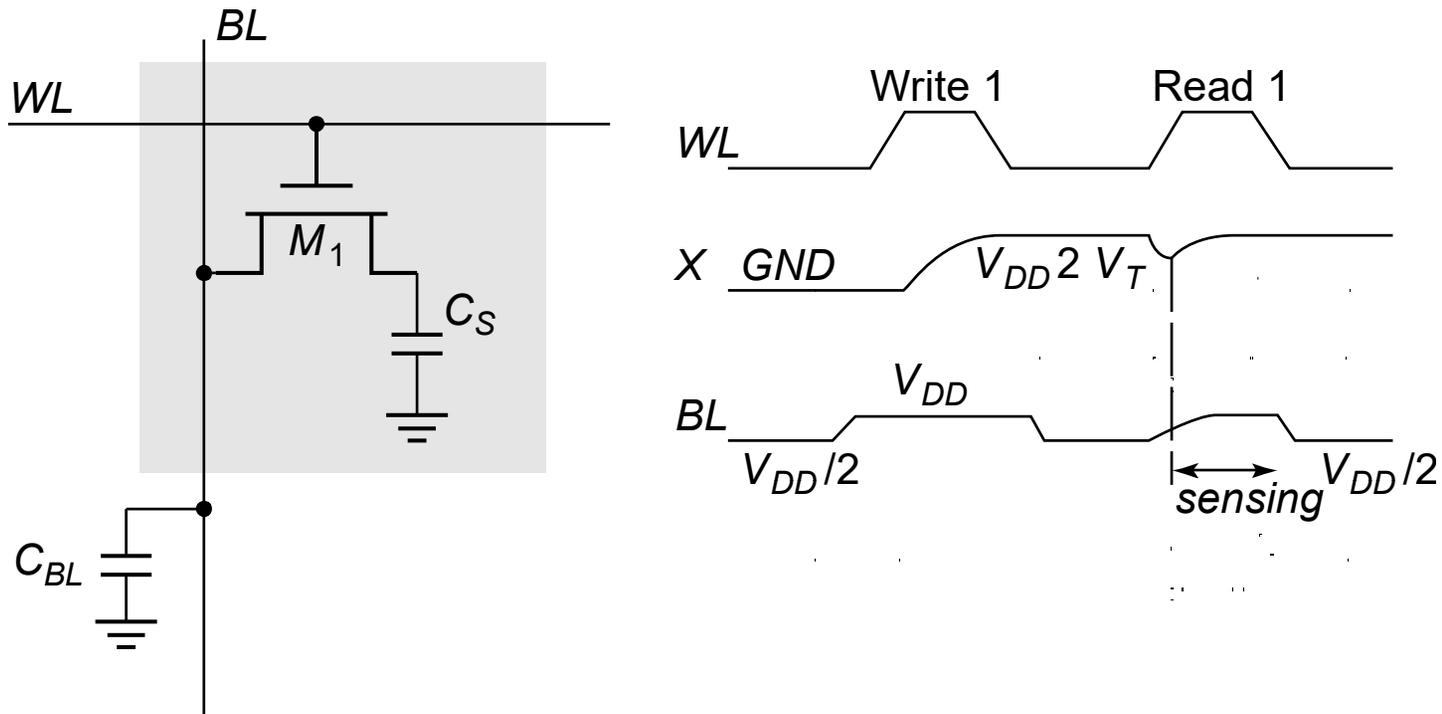
**Write:**  $C_S$  is charged or discharged by asserting WL and BL.
