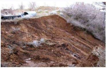
b) Translational slides occurs when the failure surface is approximately flat or slightly undulated
