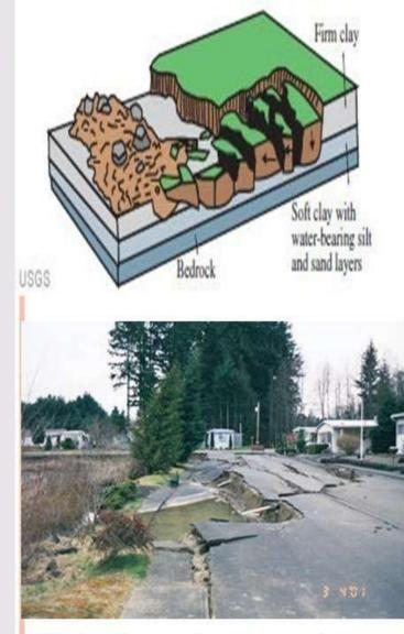
e) Lateral spreading occurs when the soil mass spreads laterally and this spreading comes with tensional cracks in the soil mass.
