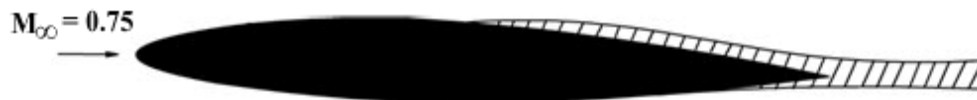
Fig.3.26 (b) M_\infty only slightly higher than M_{crit} ; shock waves are not discernible
