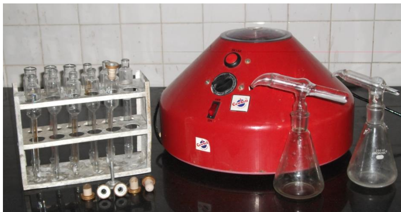
Fig. 43.1 Gerber fat testing assembly
