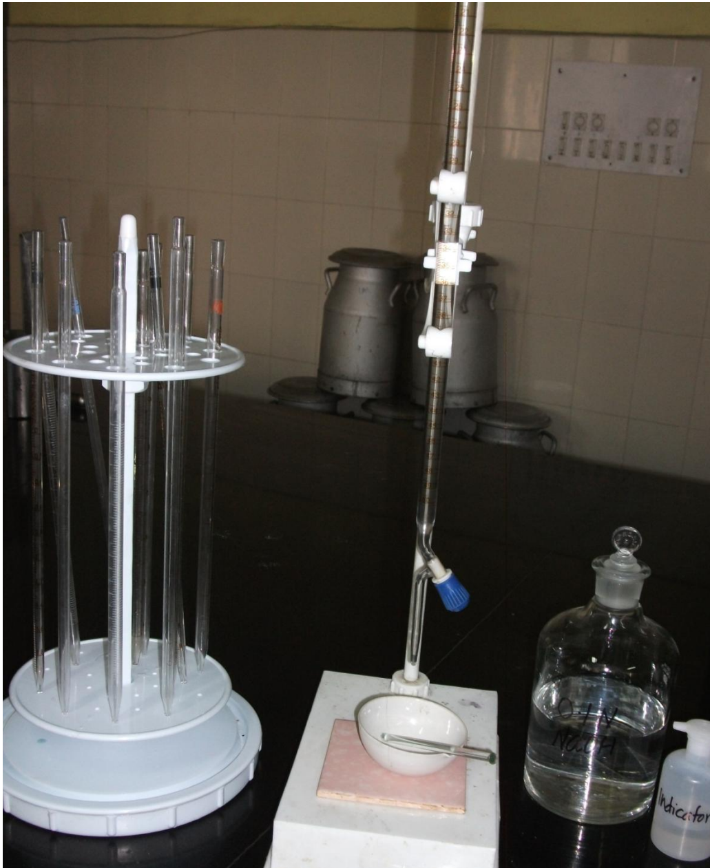
Fig. 43.3 Acidity checking assembly
