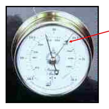
Most aneroid barometers have a needle which can be set to remember the previous reading.
