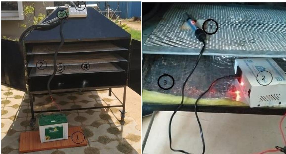
Figure 2. Experimental set up of back side of Hybrid type of Solar dryer. Figure 3. Experimental set up for night purpose
