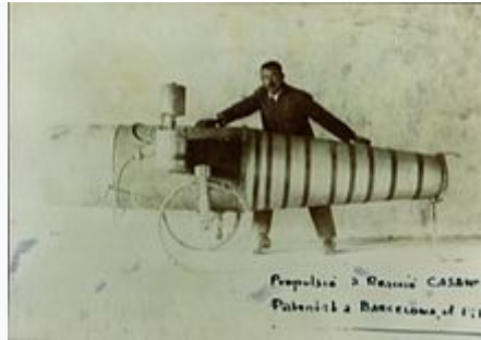
Ramon Casanova and the pulsejet engine he constructed and patented in 1917
