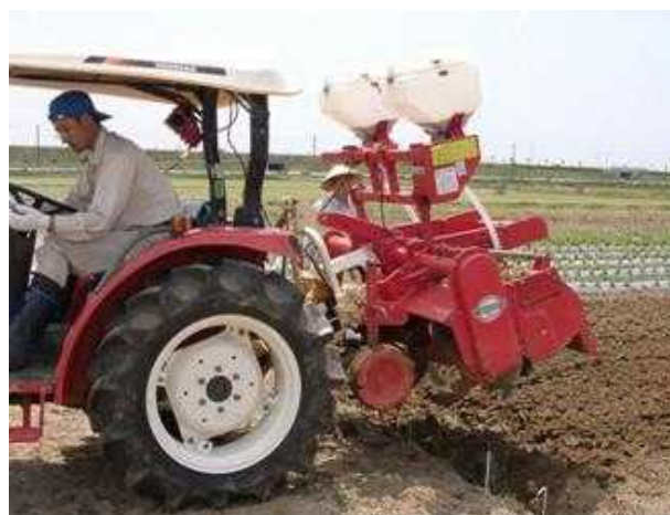
Fig.2: Fertilizer application by deep placement method
