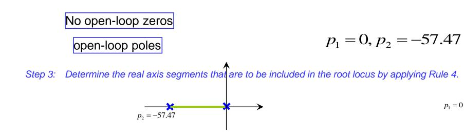
Step 4: Determine the number of asymptotes and the corresponding intersection  $\sigma_0$  and angles  $\theta_k$  by applying Rules 2 and 5.  $\sigma_0 = \frac{\sum p_i - \sum z_i}{N_p - N_z} = \frac{-57.47}{2} = -28.74$  $\begin{array}{l}
