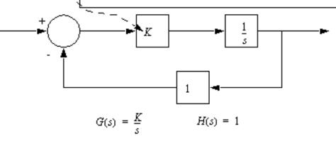
First, we must develop a transfer function for the entire control system.
