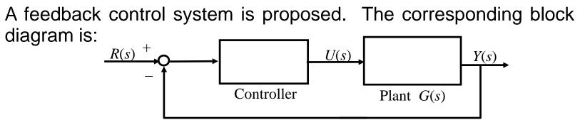
Sketch the root locus of the closed-loop poles as the controller gain K varies from 0 to  $\infty$ .
