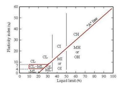
Depending on the point in the chart, fine soils are divided into clays (C), silts (M), or organic soils (O). The organic content is expressed as a percentage of the mass of organic matter in a given mass of soil to the mass of the dry soil solids. Three divisions of plasticity are also defined as follows.
