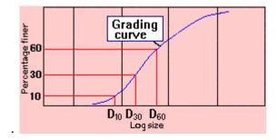
To obtain the grading characteristics, three points are located first on the grading curve.
