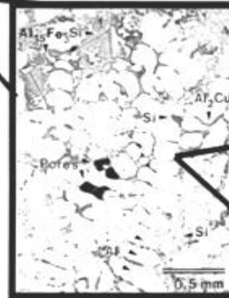
Microstructure - Dendrites & Phases ≡ 50 – 500 micrometers
