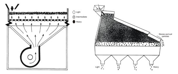
Working principle of the specific gravity separator
