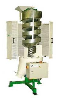
The orbit of round seed increases with speed on its flight around the axis, until it rolls over the edge of the inner flight into the outer flight where it is collected separately. The slower moving seed does not build up enough speed to escape from the inner flight. Most spirals have multiple inner flights arranged one above the other to increase the capacity.
