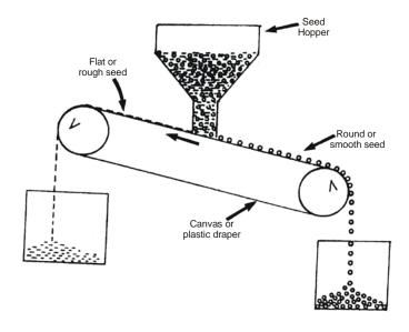
Working principle of the roll mill
