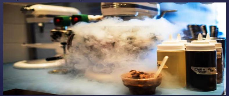
Liquid nitrogen requirement is 0.56 kg per kg of ice cream to be hardened. However, after 2 weeks storage pronounced shrinkage was evident. In few countries (viz., Sweden) ice cream cones are hardened at the rate of 11,000-16,000 per h with the help of sprayed liquid nitrogen. The cones are precooled by exhaust nitrogen in the first section and final freezing takes place in the second section.
