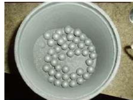
Figure 5-b An example of Grinding media for ball mill (Lead antimony-grinding media with aluminum powder)
