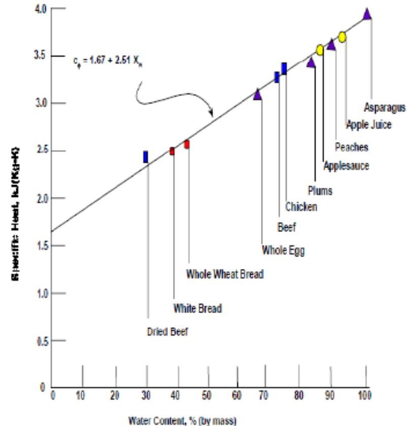
Figure 2.07. Specific heat of food products (at 0° to 20°C for meats, 4° to 32°C all others). Based upon ASHRAE data. (Courtesy of the American Society of Heating, Refrigeration and Air-Conditioning Engineers, 1989.)
