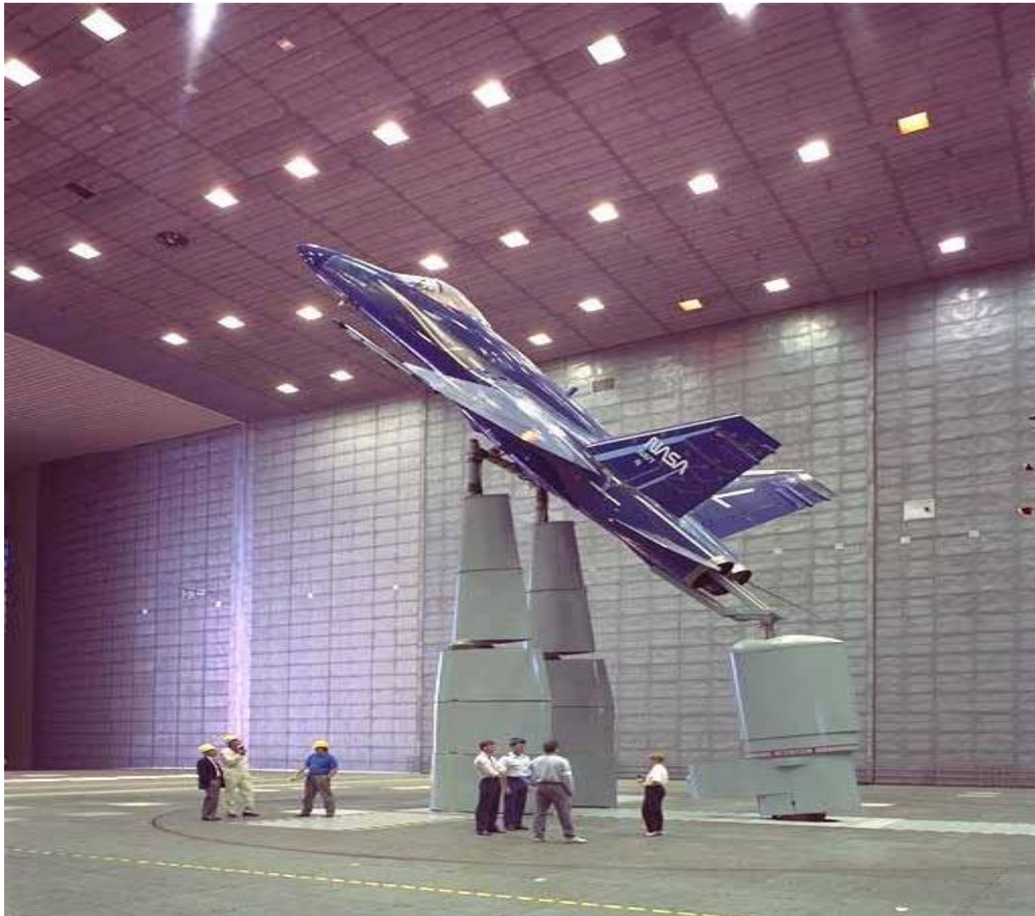
Full-Scale Test of F-18 in NASA Ames 80x120-Foot Tunnel
