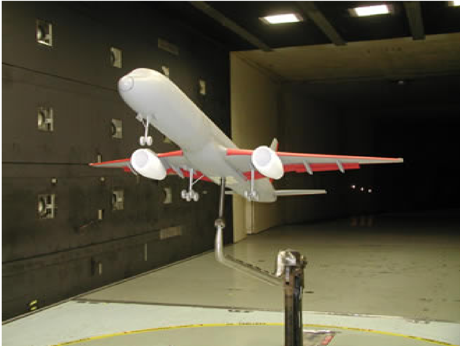
Boeing 757 Model in NASA Langley 14x22-Foot Wind Tunnel
