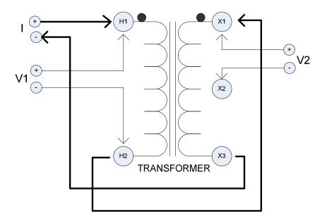
Figure 3. Measuring two windings simultaneously
