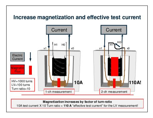
Figure 4. Amplification of magnetic flux by dual injection technique
