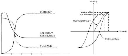
To the left: Illustration of Voltage, Current and Apparent resistance as function of time. To the right: A typical hysteresis curve for a magnetic material, e.g. transformer core. The Inductance L is proportional to the slope of the curve when current is changed
