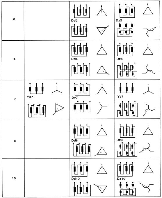
Figure 2. Alternative 3-phase Transformer Connections
