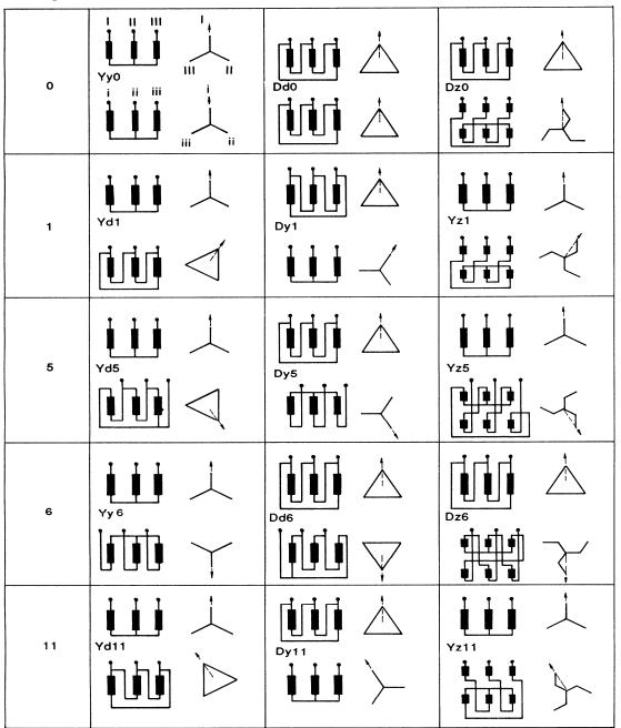
Figure 1. Common 3-phase Transformer Connections
