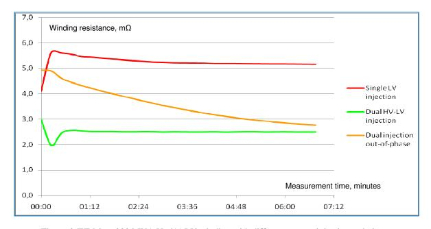
Figure 6. WRM on 200 MVA Ynd11 LV winding with different current injection techniques
