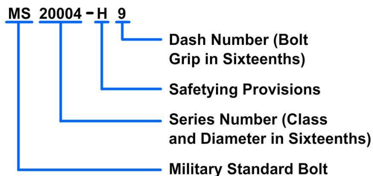
Figure 6-15 — MS bolt part number breakdown.
