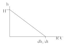
we can write the equation for a straight line to represent the rate of climb over that straight line segment.
