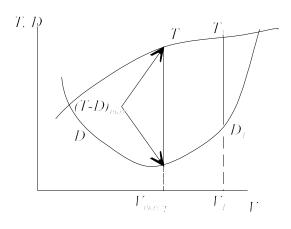
Also by trial and error, (and a pair of dividers) we can look at the differences of the two curves and determine at what speed the distance is the greatest. That speed will be the max angle of climb speed with the corresponding value of  $\gamma$  being the max angle of climb.
