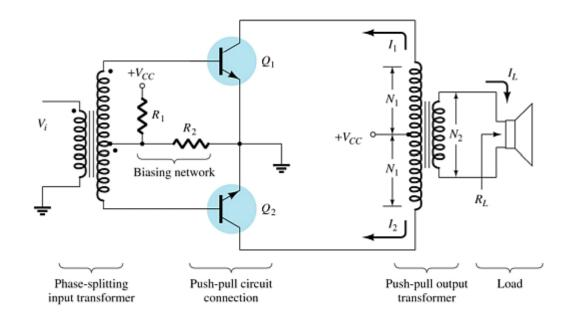
Each transistor produces one-half of an AC cycle. The transformer combines the two outputs to form a full AC cycle.
