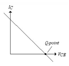
The Q-point is at 0V on the load line, so that the AC signal can only swing for one-half cycle.
