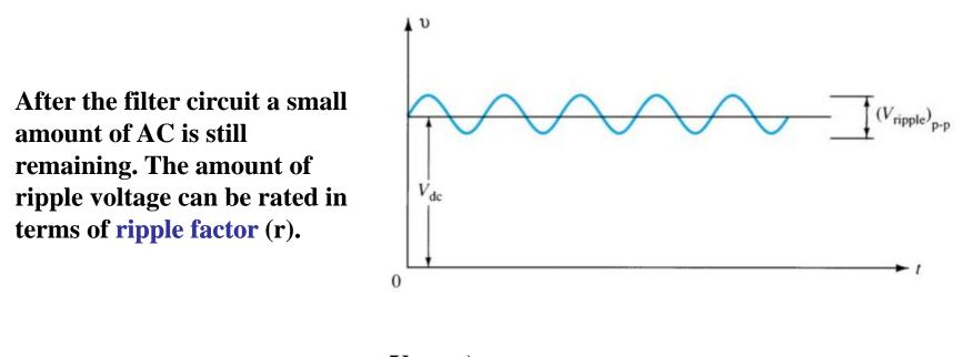
$$%r = \frac{ripple voltage (rms)}{dc voltage} = \frac{V_{r(rms)}}{V_{dc}} \times 100$$
