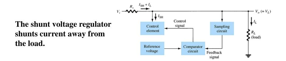
The load voltage is sampled and fed back to a comparator circuit. If the load voltage is too high, control circuitry shunts more current away from the load.
