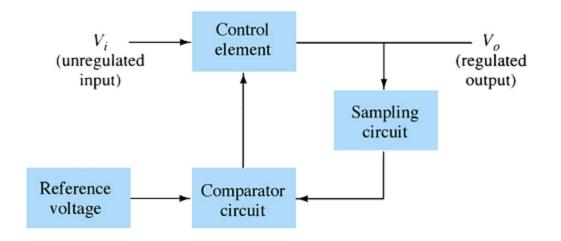
The series element controls the amount of the input voltage that gets to the output.
