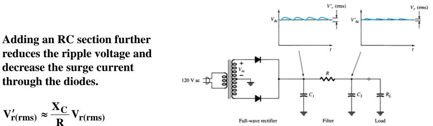
$V'_{r(rms)}$  = ripple voltage after the RC filter  $V_{r(rms)}$  = ripple voltage before the RC filter R = resistor in the added RC filter  $X_{C}$  = reactance of the capacitor in the added RC filter
