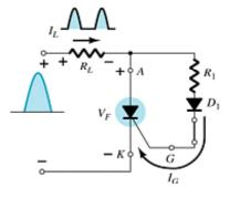
In this example, the SCR fires later—at the 90° point—on the positive half-cycle.
