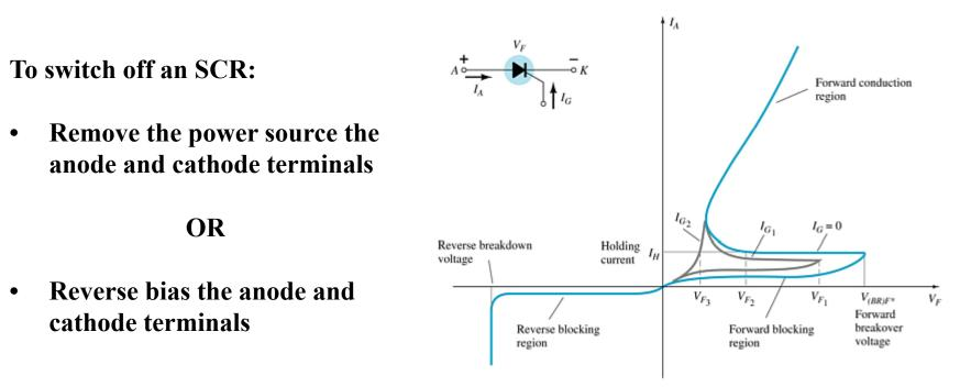
An SCR cannot be switched off by simply removing the gate voltage.
