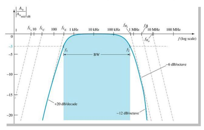
Note the *highest* lower cutoff frequency  $(f_L)$  and the *lowest* upper cutoff frequency  $(f_H)$  are closest to the actual response of the amplifier.
