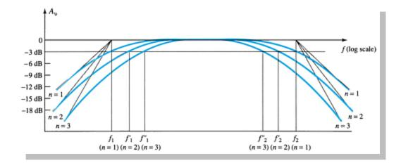
Once the cutoff frequencies have been determined for each stage (taking into account the shared capacitances), they can be plotted.
