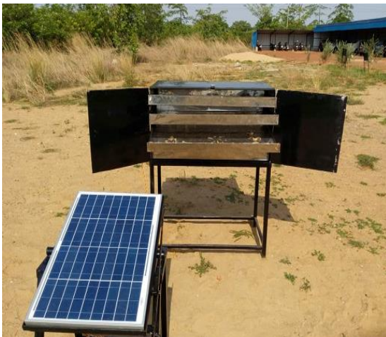
Figure 3.4. Installation of solar Dryer for the livelihood security of fisherwomen of South Odisha
