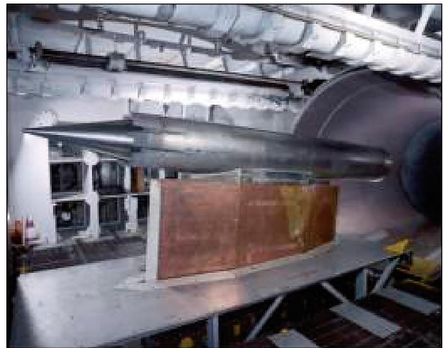
Figure 4. DCR in the HyFly configuration installed in the NASA Langley Research Center 8-ft High Temperature Tunnel.
