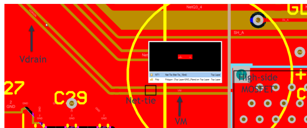
Figure 45. Net Tie High-Side MOSFET Drain
