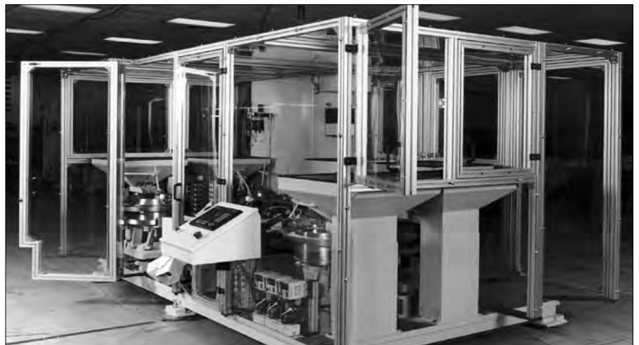
Fig. 8c: Machine guard with sliding access doors and easy to remove panels
