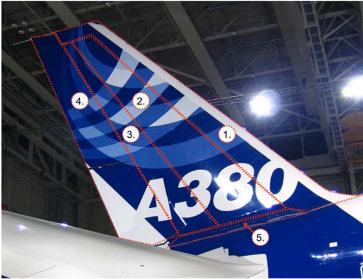
Figure 4. VTP major structural assemblies (example A380).
