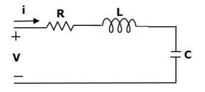
By comparing Equation 1 and Equation 3, we will get the analogous quantities of the translational mechanical system and electrical system. The following table shows these analogous quantities.
