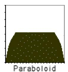
The taper of a geometric shape  $y^2 = k * x^b$ where x = distance from the apex of the shape & y = dia Specific values of b correspond to common shapes
