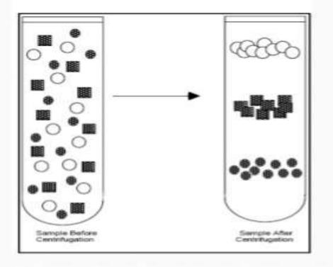
In Isopycnic centrifugation separation of particles occurs into zones on the basis of their density differences, independent of time.
