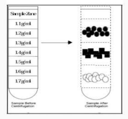
The particles will begin sedimenting in separate zones according to their size shape and density.
