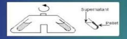
Sedimenting particles have only short distance to travel before pelleting. Shorter run time. The most widely used rotor type.
