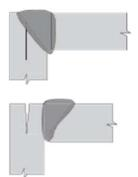
joint where there is high restraint. Special joint design is one way to minimize this defect but the best precaution is to specify materials of adequate quality and test at the receiving inspection.
