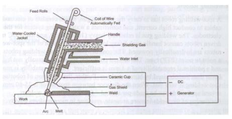
Figure 3.1 : Insert Gas Shielded Arc Welding with a Continuous Wire Fed as Electrode
