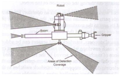
Figure 3.3 : Robot Transducers with Coverage Areas
