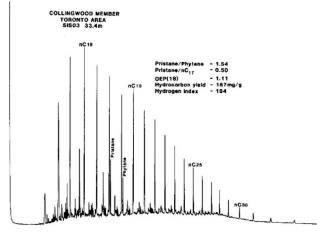
Figure 4: Saturate Fraction Gas Chromatogram – Ontario Oil Shale Formation (Collingwood Member)<sup>6</sup>
