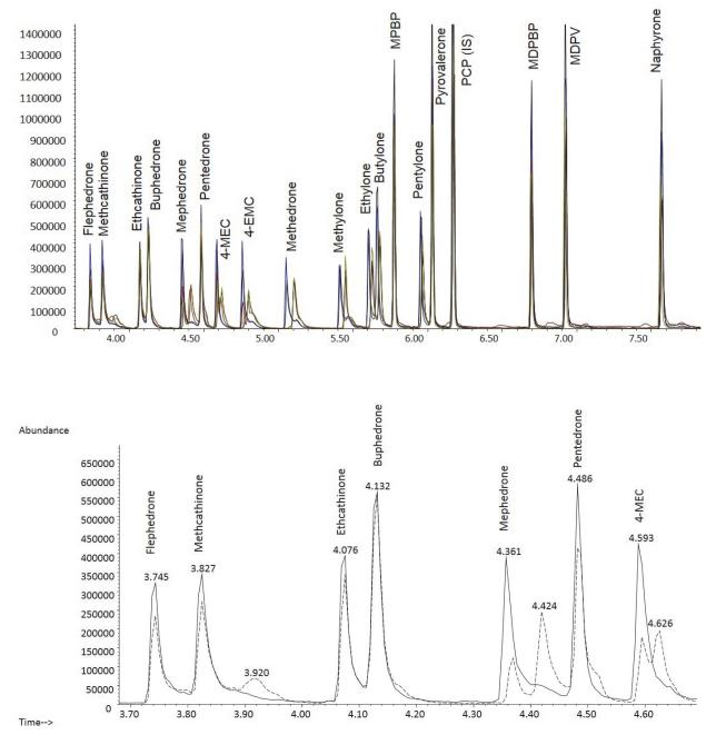
**Figure 32.** Increases in artifact peaks over 25 days at 5 day intervals (top) and a representative portion of the chromatogram showing the formation of artifacts 10 days apart (bottom).
