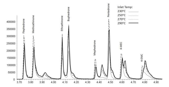
During a split injection the residence time of the sample in the injection port is very short because of the very high carrier gas flow rate through the injection liner and out of the split vent. The split ratio influences not only the quantity of sample that is introduced, but its velocity. Residence time did influence in-situ degradation. This was quantitatively evaluated
