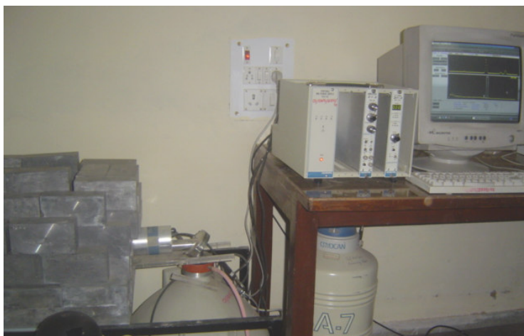
Fig. 13.12: Photographic representation of the HPGe counting set up with lead shielding and associated electronics
