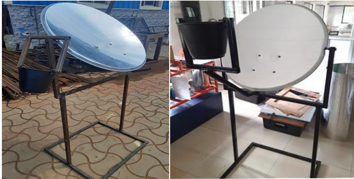
Figure 1 represents the experimental set up of solar dish type concentrator with manual operated tracking system
