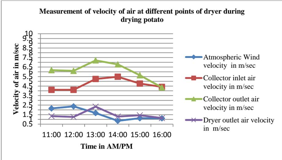
Graph 6: Measurement of velocity of solar dryer for drying potato at various points
