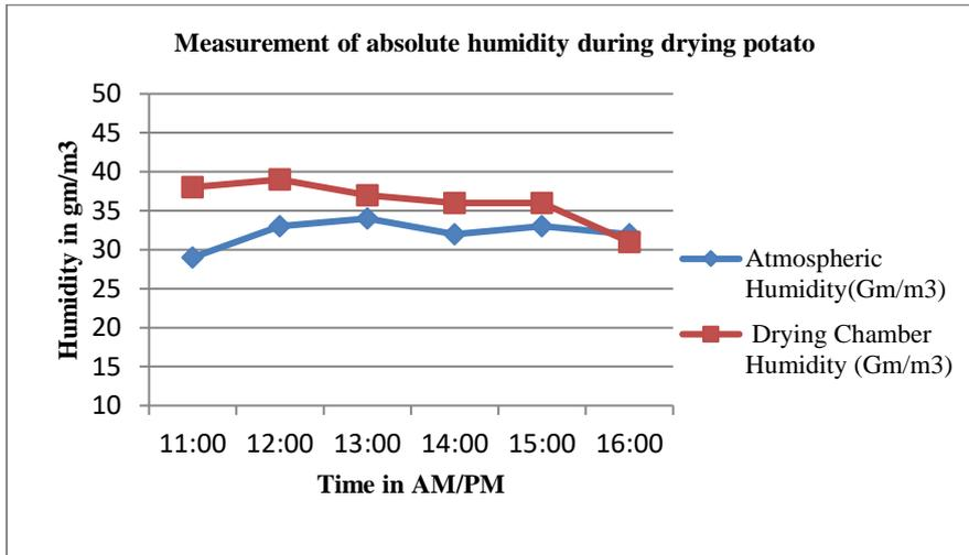
Graph 4: Absolute humidity vs. Time during drying potato
