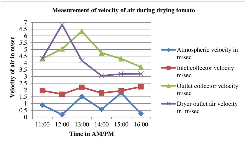
Graph 9: Measurement of velocity of solar dryer for drying tomato at various points
