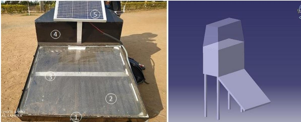
Figure 1. Experimental set up of front side of Hybrid type of Solar dryer.
