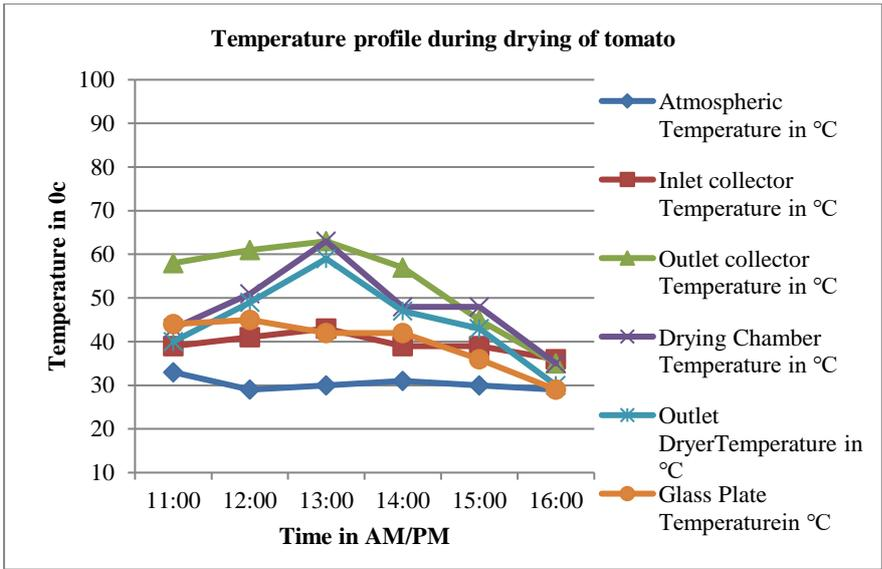
Graph 8: Measurement of temperature during drying tomato
