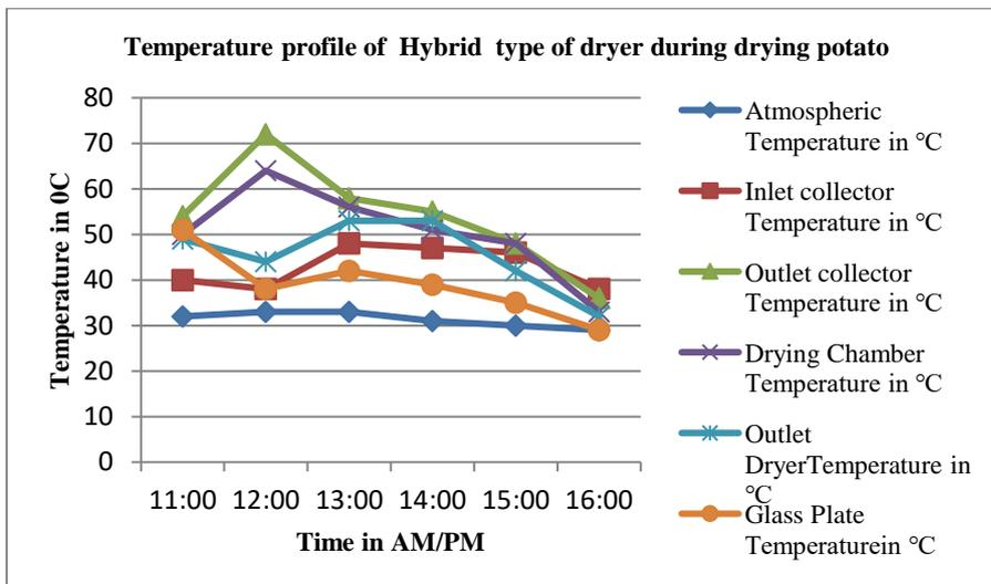
Graph 5: Measurement of temperature during drying potato
