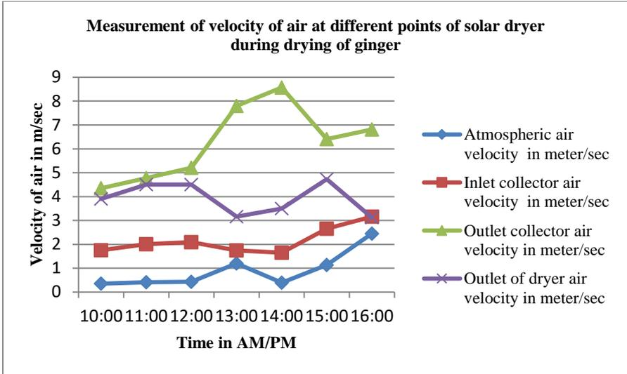
Graph 3: Measurement of velocity of air of solar dryer for drying ginger
