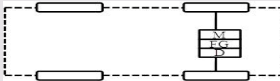
Figure 3c: EV configuration with clutch, gearbox and differential
