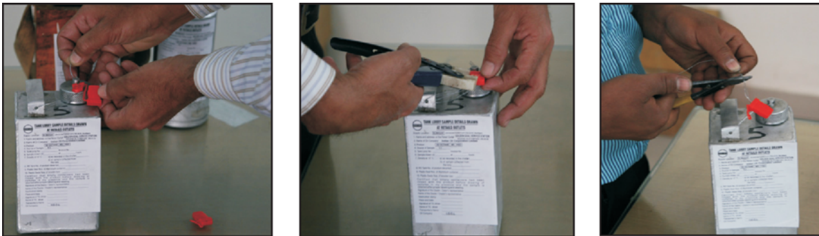
Figure 11.8 (left to right): Method of sealing the sample container
